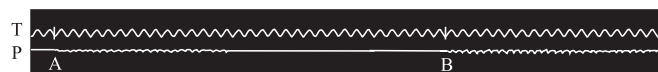
Fig. 1. Stylized versions of the phonautograph and noematachograph, and the noematachograph from Donders (1868) showing the speech waves of two persons (P), the sound wave of a tuning fork (T), and vertical marks indicating the speech onsets (A and B) of the persons.
